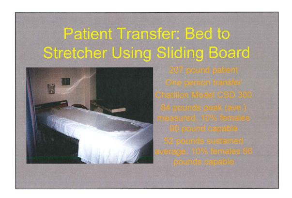
The second approach reviewed was the use of a sliding board. This device is a polypropylene board with hand holds cut out, being approximately 22"x72"x3/16" with corner cutouts. It provides a solid surface with a lower coefficient of friction than the draw sheet.
