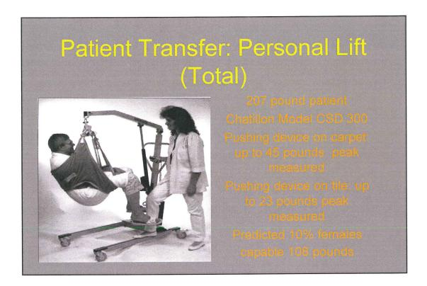
The use of devices for performing total lifts, such as the one shown here, can be helpful in reducing the physical demand for transfers from bed to chair, floor to bed, floor to chair, and others. One of the concerns with these devices, which often come equipped with power lifts but not power push/pull, are the forces required with pushing/pulling.
